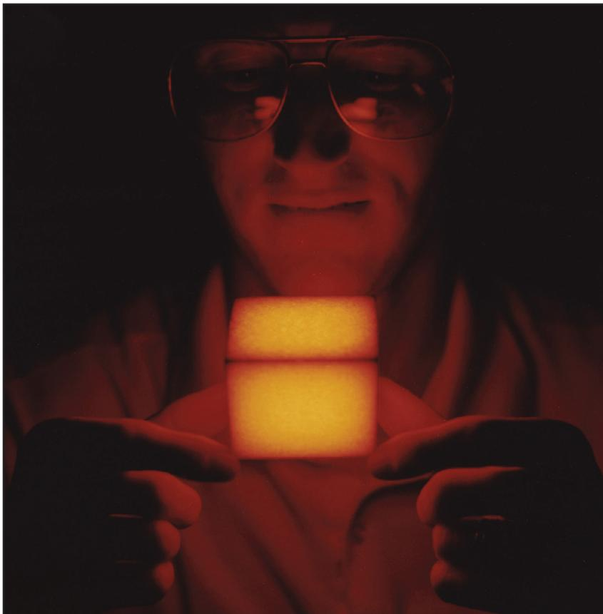
**T**his photograph shows a white-hot cube of a silica fiber insulation material, which, only seconds after having been removed from a hot furnace, can be held by its edges with the bare hands. Initially, the heat transfer from the surface is relatively rapid; however, the thermal conductivity of this material is so small that heat conduction from the interior [maximum temperature approximately  $1250^{\circ}\text{C}$ ] is extremely slow.
