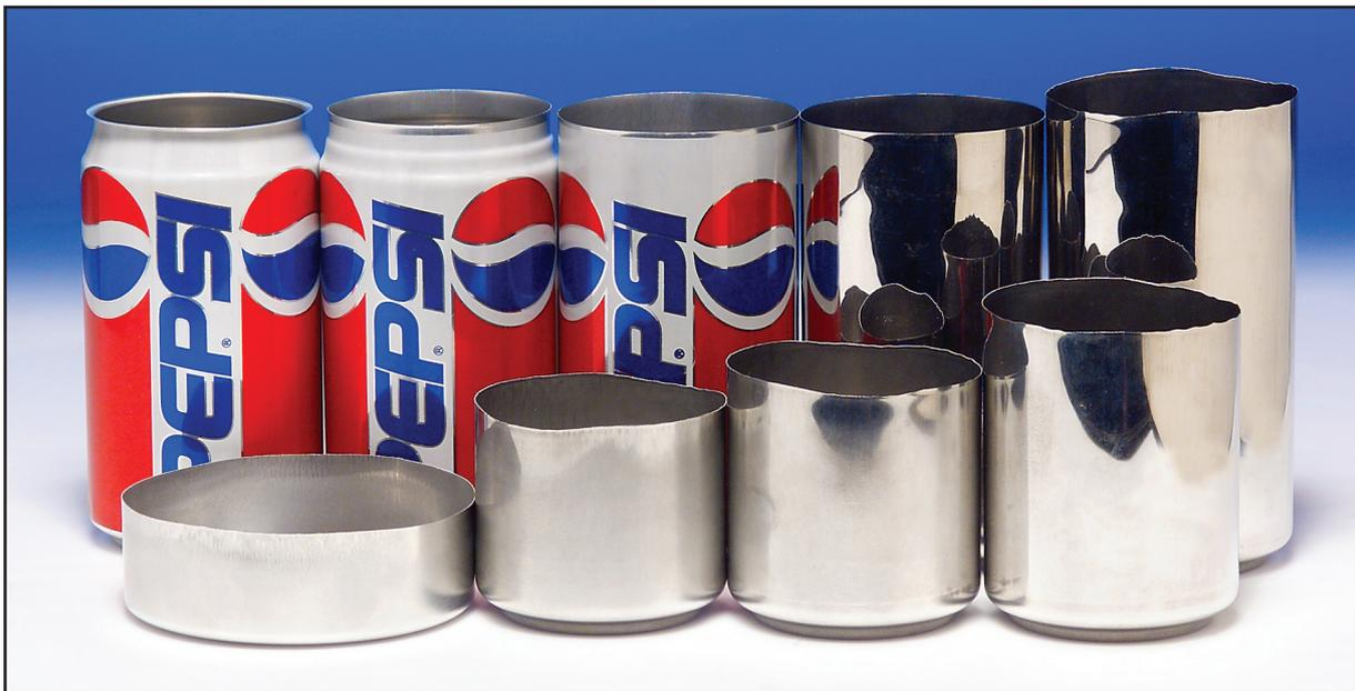
**T**his photograph shows the aluminum beverage can in various stages of production. The can is formed from a single sheet of an aluminum alloy. Production operations include drawing, dome forming, trimming, cleaning, decorating, and neck and flange forming. (PEPSI is a registered trademark of PepsiCo, Inc. Used by permission.)
